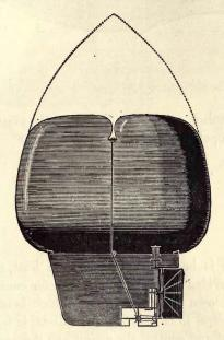
to the upper part of the balloon is drawn down when the gas is being withdrawn, for the purpose of preventing damage being caused to the balloon whilst making the descent.
